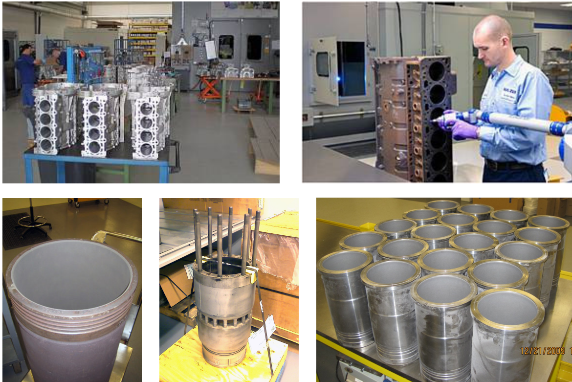
Figure 8: upper left: SUMEBore coating shop in Wohlen with a small series aluminum 4-cylinder block, upper right: SUMEBore shop in Westbury with a 6-cylinder cast iron block for remanufacturing, lower row: 4-stroke and 2-stroke locomotive engine liner and liners from an industrial gas engine
