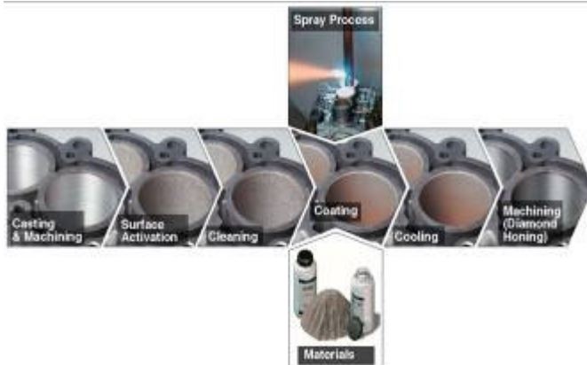
Figure 2: Schematic representation of the SUMEBore process (from left to right, including honing)
